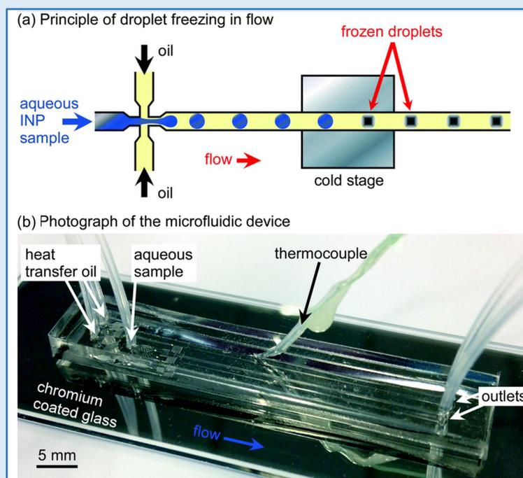
Figure 6 (a) Droplet freezing in flow. (b) Photograph of LOC-NIPI. (Tam et al., 2020) [4]
