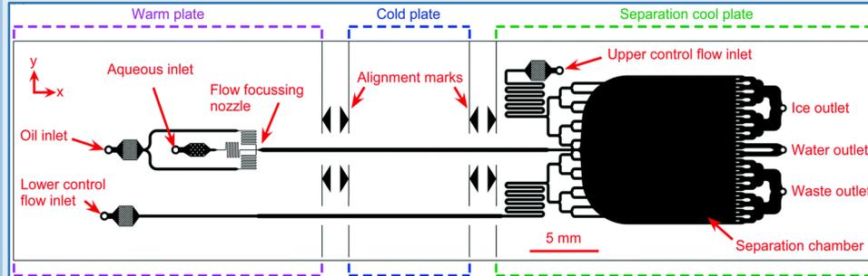
Figure 3 Design of the microfluidic chip in LOC-NIPI. (Porter et al., 2020) [5]
