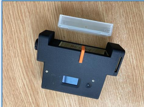
Figure 2 Handheld electrostatic precipitator and box containing collection slides
