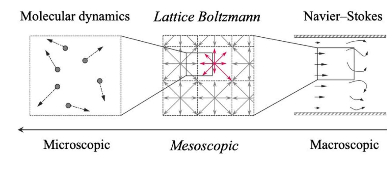
$$f_i(\underline{x} + \delta c_i, t + \delta t) = f_i(\underline{x}, t) + \Omega_i$$
