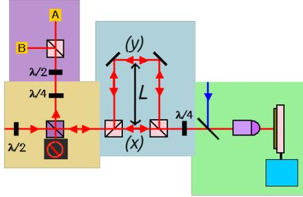
Figure 1: diagram of my Sagnac interferometer, the design is based on [14], just like in [15], the Sagnac time delay is at 500ps however I have my apparatus set up in such a way that the time delay is easily adjustable
