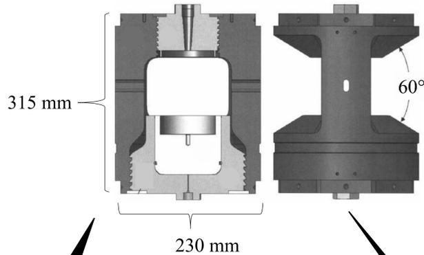
Size Kept to a Minimum  $\rightarrow$  Lightweight ( $\approx 50 \text{ kg}$ ) and Portable
