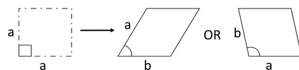
All transformations are equally likely, therefore different regions of the  $\text{Cd}_3\text{As}_2$  crystal may transform into different monoclinic structures. This behaviour will lead to domains with walls between them. Upon transition back to a sample wide tetragonal structure, domain walls will leave dislocations/defects in the crystal. Applying this simple idea allows the observed behaviour to be explained by the Drude model, from which we have
