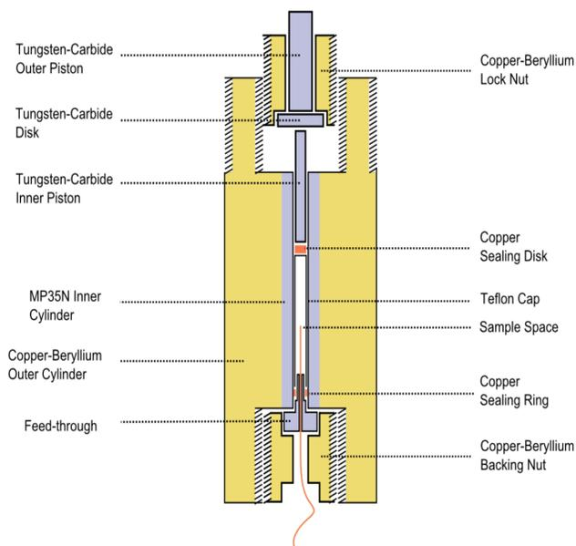
Four-point electrical transport measurements of Manganin (a),  $\text{Cd}_3\text{As}_2$  (b) and bismuth (c) samples were made via an electrical feedthrough. The samples were contained within a Teflon cap filled with glycerin; the pressure transmitting medium.
