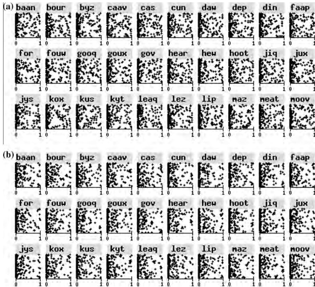
Fig. 7. Sparseness plots of the network trained on lists of words taken from the (a) small and (b) large vocabularies. Each plot refers to a word rather than a hidden unit and only the plots of the words from the small vocabulary are presented. Each cross refers to a hidden unit, with level of activation along the x-axis (from 0 to 1) and hidden unit number (1–200) organized along the y-axis (200 crosses per plot).
