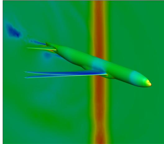
Figure 4 SVM simulation of NCRM encountering a 18.288 m '1-cosine' gust
