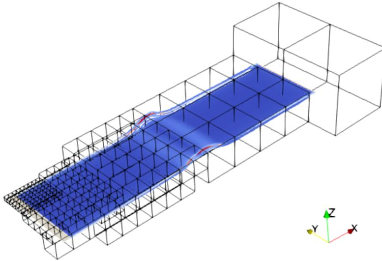
**Figure 1** Octree box structure for a point close to the wing-tip. Solution show a generic UAV wing plus wake post 1-cosine gust impact.
