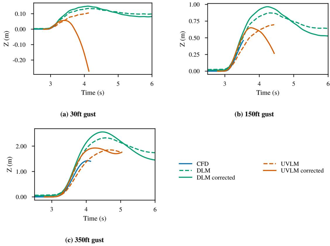
**Figure 10** Change in altitude for the free NCRM calculated using steady corrections
