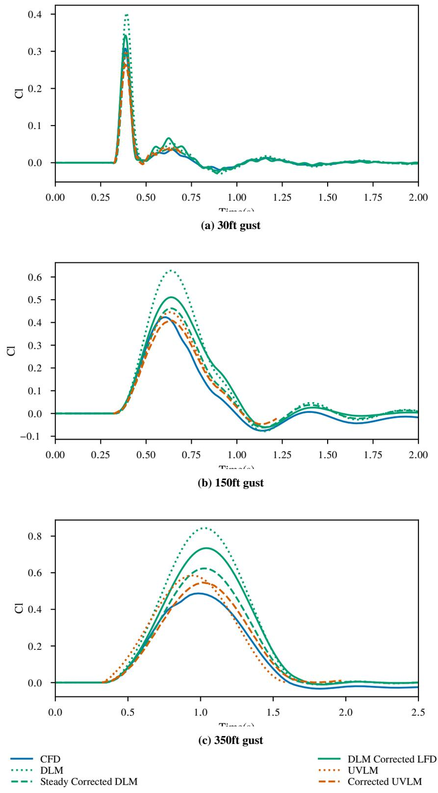
Figure 6 Gust response for aeroelastic generic UAV wing
