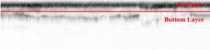
Figure 5. GPR processing example: division into layer regions
