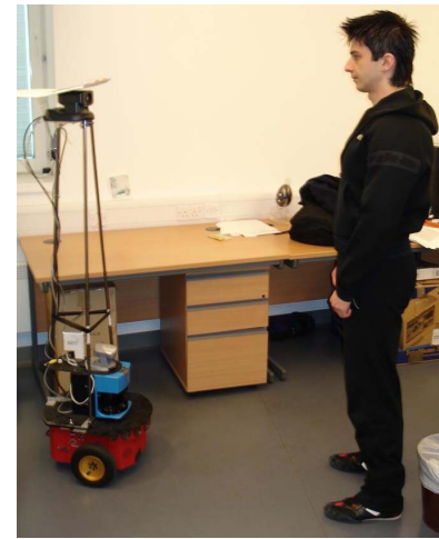
Fig. 3. Mobile robot with laser and camera.
