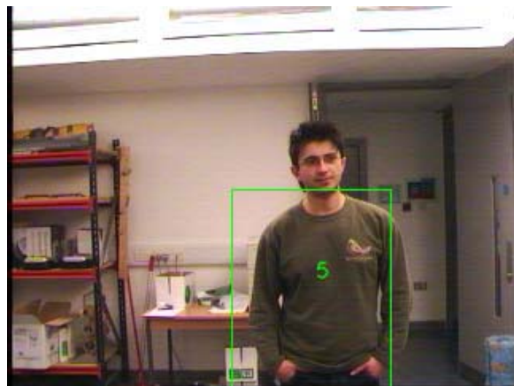
Fig. 1. Region from where histograms are extracted and then compared to that one in the database. The number 5, which indicates the record inside the current database, is centred on the sub-region where the histogram matches best, namely at the pixel location (u_c, v_c) .
