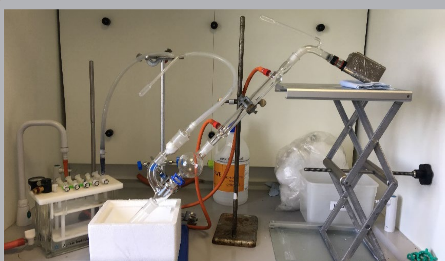
Fig 2: Vaping simulation apparatus. E-cigarette is connected via glass tubing to vacuum pump with adjustable pressure. Condenser and ice bath aid collection of liquefied vapour and aerosol.
