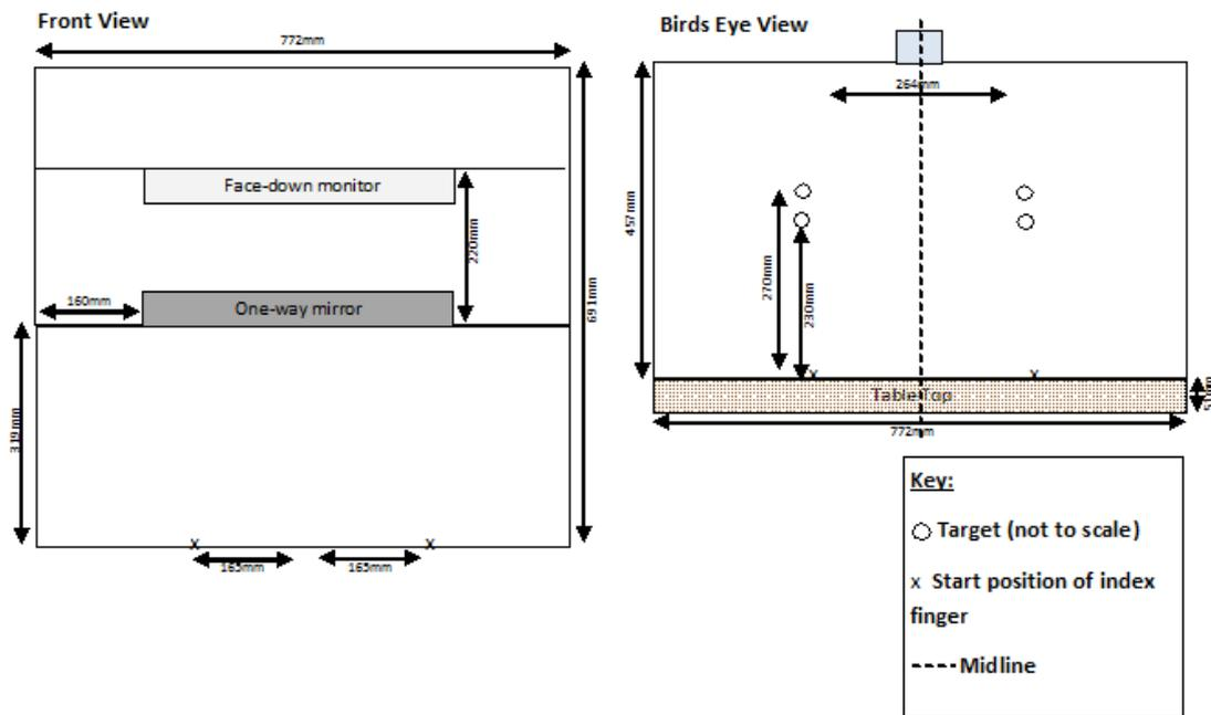
**Fig.1.** Simplified diagram of the MIRAGE VR system, displaying measurements and distances. All to scale (except target size).
